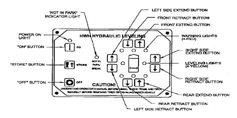
To extend, press the "ON" button on the HWH control panel. The "POWER ON" light will illuminate. Place pads under the jacks, if necessary, at this time. A lit yellow "LEVEL" light indicates that the end, side, or corner is low. Push an "EXTEND" (up arrow) button to extend the jack pairs according to the lit yellow lights. Always level the vehicle from side to
