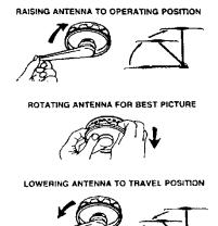
The antenna must be lowered before moving the vehicle. To lower, rotate the directional handle until the pointer is aligned with the pointer on the ceiling plate. Turn the elevating crank (counter-clockwise) in the "DOWN" direction, about 13 turns, or until some resistance to turning is noticed. The antenna is now locked and in the travel position. Your unit may be equipped with one exterior antenna jack and two interior antenna jacks.
