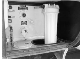
When replacing the filter, make certain the rubber "O-Ring" seal is properly positioned in its groove in the cartridge housing. An improperly seated or missing seal will cause leakage around the perimeter of the filter housing. Use caution not to over tighten the canister when attaching it back to the housing.
