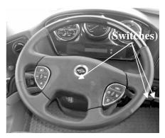
The right side bottom switch moves the brake and throttle pedals under the dash. This allows for greater flexibility in seating position, as well as improved individual access to the pedals.
