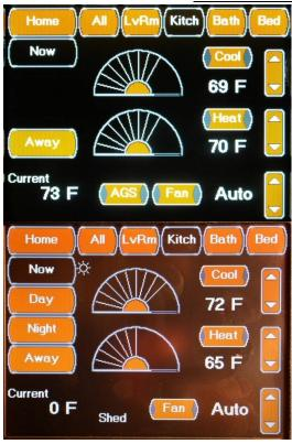
The Climate "Kitch" Screen displays the status and control the Kitchen Zone (Zone2) HVAC system.
