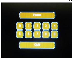
The Password Access Screen is to provide access to advanced system configuration screens. These screens contain control settings that should only be changed by qualified individuals.
