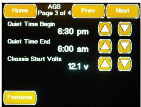
The third Autogen Configuration screen is accessed by pressing the Next Button located on the second Autogen Configuration screen or by pressing the "Prev" Button located on the fourth Autogen Configuration screen.
