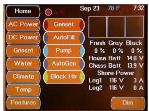
All control functions can be accessed by pressing one of the Buttons on the Home Screen. The Home Screen also displays system status and warnings in order of priority.
