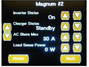
The first Magnum2 Setting Screen1 is only available on a dual inverter system (King Aire) and configures the following settings:
