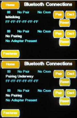
The Bluetooth Connections screen(s) is accessed by pressing the Bluetooth Connections Button located on the Features Configuration screen .This screen displays connection information for two Bluetooth Modules and allows you to change the following settings:
