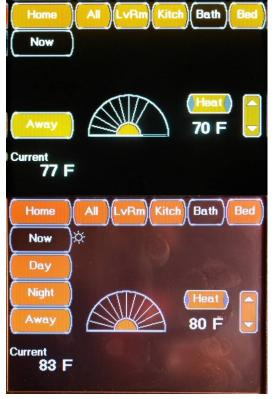
The Climate "Bath" Screen displays the status and controls the Bathroom Zone (Zone3) HVAC Oasis heating system. Pressing the Heat Button activates the zone's HVAC function. The set points can be changed by pressing the associated up and down arrows or by dragging the associated circular temperature wheel to the desired set point.
