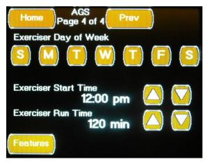
The fourth Autogen Configuration screen is accessed by pressing the Next Button located on the third Autogen Configuration screen. This screen allows you to change the following settings:
