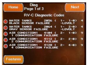
The first Systems Diagnostics Screen is accessed by pressing the System Diagnostic Button located on the Features Screens or from the "Prev" Button located on second Systems Diagnostics Screen. This Screen displays any system faults present on the control system.
