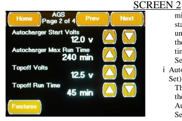
The second Autogen Configuration screen is accessed by pressing the Next Button located
