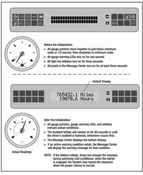
Figure 1-2 System Initialization Sequence
