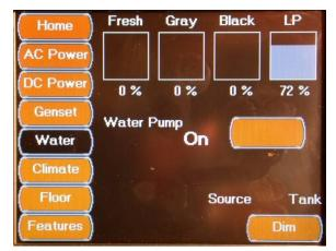
The Water Screen for a coach equipped with an LP tank, displays and controls the same functions as the All Electric Water Screen with the addition of the LP tank % full status.
