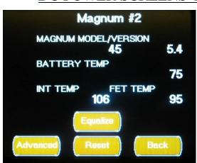
The DC Power (Settings) Magnum2 Status Screen is only available on a dual inverter system (King Aire) and displays the following Status Values:
