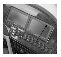
mounted on the rear cap of your motorhome faces down and back to help you when backing the unit, when observing traffic in transit, or when checking on a vehicle you are towing behind your unit. This camera comes on automatically any time your RV transmission is in reverse. It can also be manually selected using the "Camera Select" button on the dash switch panel below the monitor.
