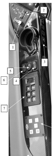
1. ATC Switch turns the Automatic Traction Control system on and off.
