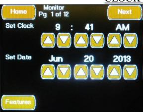
This screen provides a means to set the system time. The system time and date are set by pressing the associated up and Down Buttons
