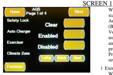
The first Autogen Configuration screen is accessed by pressing the Autogen Configuration
