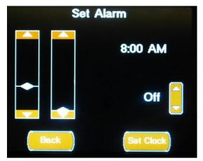
The Set Alarm screen is accessed from the Clock screen. The Alarm time value is set by means of the two slider bars and enabled from the Up/Down Button. This screen also provides access to setting the system time via the Set Clock Button.
