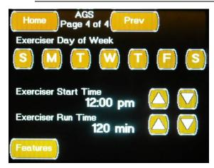
The fourth Autogen Configuration screen is accessed by pressing the Next Button located on the third Autogen Configuration screen.
