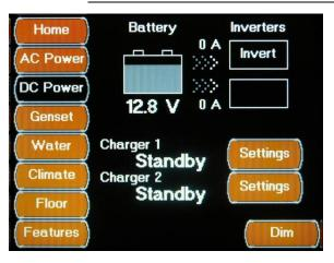
The Main DC Power Screen displays the Inverter(s) / Charger(s) status and allows access to the Operator Accessible Magnum Setting Screens
