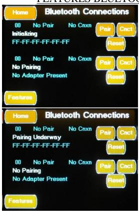
The Bluetooth Connections screen(s) is accessed by pressing the Bluetooth Connections Button located on the Features Configuration screen .This screen displays connection information for two Bluetooth Modules and allows you to change the following settings:
