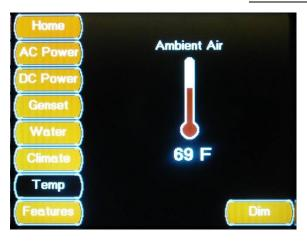
The Temp screen is accessed by pressing the Temp Button located on the Home Screen. This screen displays the Outside Air Temperature. The Temp Button is only available on systems without the optional Floor Heat.
