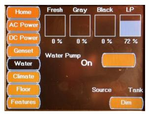
The Water Screen for a coach equipped with an LP tank, displays and controls the same functions as the All Electric Water Screen with the addition of the LP tank % full status.
