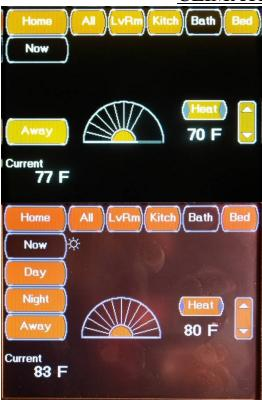
The Climate "Bath" Screen displays the status and controls the Bathroom Zone (Zone3) HVAC Oasis heating system.
