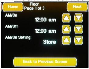
The first Floor Heat Configuration screen is accessed by pressing the Floor Heat Configuration Button located on the Features Configuration Screen or by pressing the "Prev" Button located on the second Floor Heat
