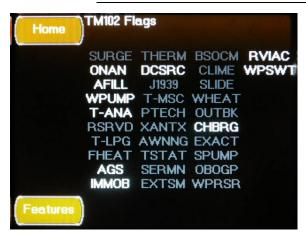
The TM102 Flags screen is accessed by pressing the TM102 Configuration Button located on the Features Configuration Screen. This screen displays the active system functions
