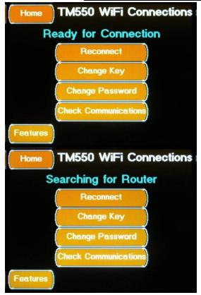
The TM550 WiFi Connections screens are accessed by pressing the TM550 WiFi Connections Button located on the Features Configuration screen .These screens display connection information for the TM550 WiFi Module and allows you to configure the following settings:
