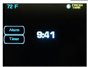
The Clock display screen is accessed by pressing the Clock Button located on the Features Screens. This Screen displays the system time and provides access to the Alarm and Timer functions.
