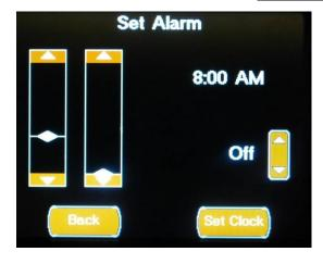
The Set Alarm screen is accessed from the Clock screen. The Alarm time value is set by means of the two slider bars and enabled from the Up/Down Button.
