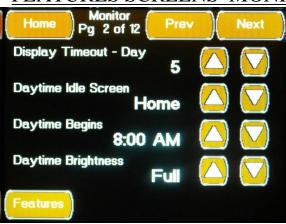
The second Monitor Configuration Screen is accessed by pressing the Next Button located on the first Monitor Configuration Screen or from the "Prev" Button located on third Monitor Configuration Screen. This Screen allows you to set the Day Time Display Setting by pressing the associated Up and Down Buttons
