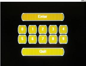
The Password Access Screen is displayed to provide access to advanced system configuration screens. The advanced configuration screens contain control settings that should only be changed by qualified individuals. Changing these control settings to an improper setting can adversely affect the operation of the control system and may cause damage to the coach
