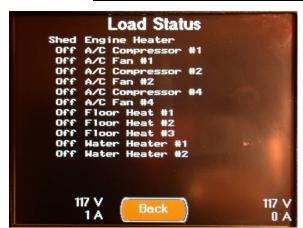
The Load Status Screen displays the Load Shed status of all the AC powered devices that are controlled by the control system. This screen also displays the AC voltage and amperage usage for both power legs. The Back Button returns you to the AC Power Screen.
