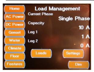
The Load Management Screen displays the Shore Power Phase setting (Single Phase 30 Amps and less Service, Dual Phase 50 Amp Service) and allows you to change between the phase selections using the Change Button. The current Amp draw is displayed for both Power Legs on this screen. The Load Status screen is selected from the Loads Button. The Load Settings Screen is selected from the Settings Button.
