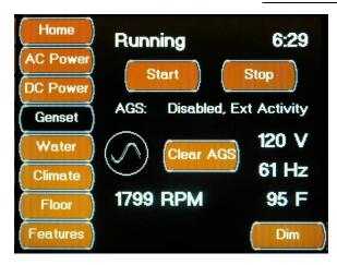
The Genset Screen displays the current Generator Status and control system run time.
