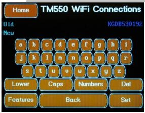
The TM550 WiFi Module Change Password Screen is accessed by pressing the Change Password Button located on the WiFi Connections Screen. This screen allows the module password to be changed.
