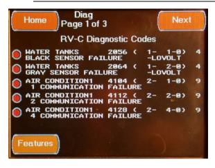
The first Systems Diagnostics Screen is accessed by pressing the System Diagnostic Button located on the Features Screens or from the "Prev" Button located on second Systems Diagnostics Screen. This Screen displays any system faults present on the control system.
