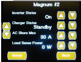
The first Magnum2 Setting Screen1 is only available on a dual inverter system (King Aire) and configures the following settings:
