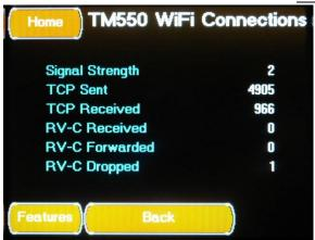
The TM550 WiFi Module Check Communications Screen is accessed by pressing the Check Communications Button located on the TM550 WiFi Connections Screen. This screen displays the TM550 WiFi Module Communications Information.
