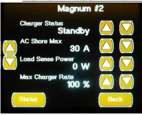
The second Magnum2 Setting Screen2 is only available on a dual inverter system (King Aire) and configures the following settings:
