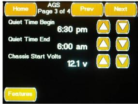
The third Autogen Configuration screen is accessed by pressing the Next Button located on the second Autogen Configuration screen or by pressing the "Prev" Button located on the fourth Autogen Configuration screen.
