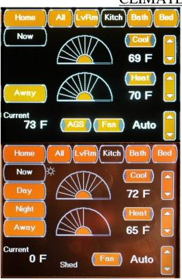
The Climate "Kitch" Screen displays the status and control the Kitchen Zone (Zone2) HVAC system.
