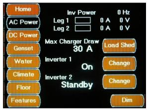
The AC Power Screen displays the AC Power Source, Line Voltage and Current (Amperage) usage, as well as, the AC Line Frequency (Hz).
