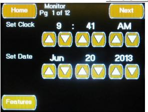
This screen provides a means to set the system time. The system time and date are set by pressing the associated up and Down Buttons
