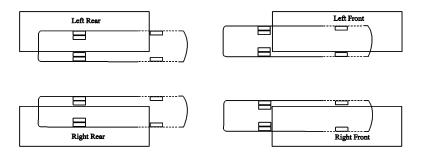
The recommended procedure to weigh a motorhome accurately is on individual corner scales. Since these are not always available, below is a diagram of how to weigh a motorhome on a typical truck scale.
