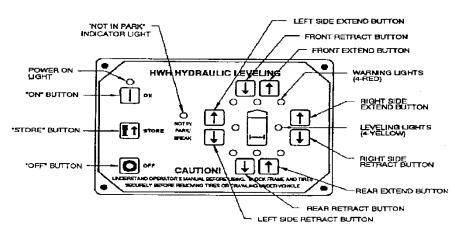
To extend, press the "ON" button on the HWH control panel. The "POWER ON" light will illuminate. Place pads under the jacks, if necessary, at this time. A lit yellow "LEVEL" light indicates that the end, side, or corner is low. Push an "EXTEND" (up arrow) button to extend the jack pairs according to the lit yellow lights. Always level the vehicle from side to
