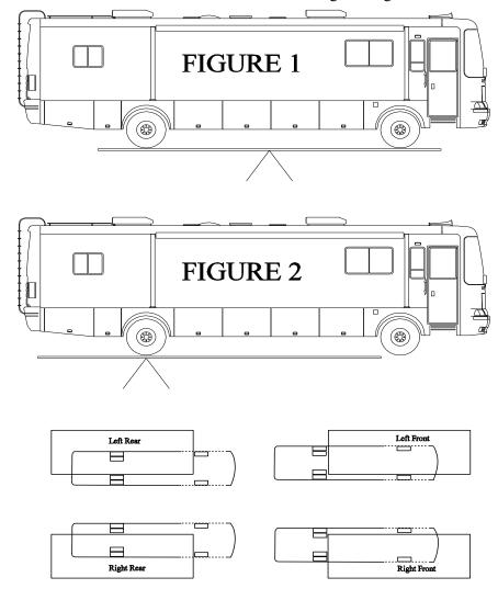
The recommended procedure to weigh a motorhome accurately is on individual corner scales. Since these are not always available, above is a diagram of how to weigh a motorhome on a typical truck scale.
