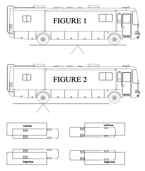
The recommended procedure to weigh a motorhome accurately is on individual corner scales. Since these are not always available, below is a diagram of how to weigh a motorhome on a typical truck scale.
