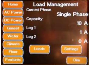
The Load Management Screen displays the Shore Power Phase setting (Single Phase 30 Amps and less Service, Dual Phase 50 Amp Service) and allows you to change between the phase selections using the Change Button. The current Amp draw is displayed for both Power Legs on this screen. The Load Status screen is selected from the Loads Button. The Load Settings Screen is selected from the Settings Button.
