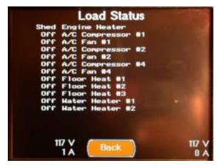
The Load Status Screen displays the Load Shed status of all the AC powered devices that are controlled by the control system. This screen also displays the AC voltage and amperage usage for both power legs. The Back Button returns you to the AC Power Screen.
