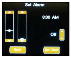
The Set Alarm screen is accessed from the Clock screen. The Alarm time value is set by means of the two slider bars and enabled from the Up/Down Button. This screen also provides access to setting the system time via the Set Clock Button.
