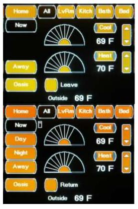
The Climate Screens are used to display the status and control functions for the HVAC system.
