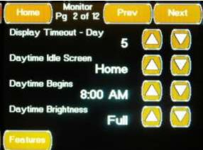
The second Monitor Configuration Screen is accessed by pressing the Next Button located on the first Monitor Configuration Screen or from the "Prev" Button located on third Monitor Configuration Screen. This Screen allows you to set the Day Time Display Setting by pressing the associated Up and Down Buttons
