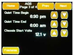
The third Autogen Configuration screen is accessed by pressing the Next Button located on the second Autogen Configuration screen or by pressing the "Prev" Button located on the fourth Autogen
