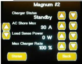
The second Magnum2 Setting Screen2 is only available on a dual inverter system (King Aire) and configures the following settings:
