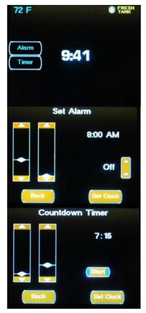
The Clock Screen is accesses by pressing the Clock Button from The Features Screen.
