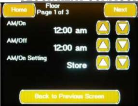
The first Floor Heat Configuration screen is accessed by pressing the Floor Heat Configuration Button located on the Features Configuration Screen or by pressing the "Prev" Button located on the second Floor Heat Configuration screen.
