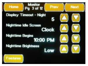
The third Monitor Configuration Screen is accessed by pressing the Next Button located on the second Monitor Configuration Screen or from the "Prev" Button located on fourth Monitor Configuration Screen. This Screen allows you to set the Night Time Display Settings by pressing the associated Up and Down Buttons
