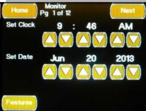
The first Monitor Configuration Screen is accessed by pressing the Monitor Configuration Button located on the Features Screens or from the "Prev" Button located on second Monitor Configuration Screen. This Screen allows you to set the system time and date by pressing the associated up and Down Buttons
