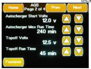
The second Autogen Configuration screen is accessed by pressing the Next Button located
