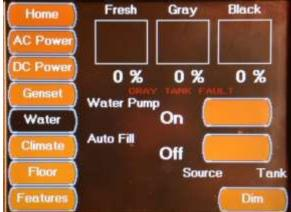
The Water Screen on coaches equipped with the All Electric option displays the Fresh and Holding Tanks volume % full status. This screen also displays tank related faults, if any. The Water Pump Button turns the Water Pump on and off. The Auto Fill Button turns the Auto Fill function on and off.
