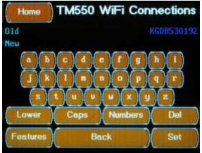
The TM550 WiFi Module Change Password Screen is accessed by pressing the Change Password Button located on the WiFi Connections Screen. This screen allows the module password to be changed.
