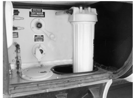
Insert the new filter cartridge, positioning it so the opening in the bottom of the filter seats on the molded ring at the bottom of the canister. Reattach the canister to the filter housing by rotating the canister in a counter clockwise direction.
