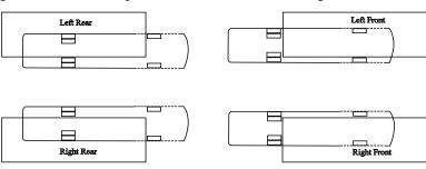
The recommended procedure to weigh a motorhome accurately is on individual corner scales. Since these are not always available, above is a diagram of how to weigh a motorhome on a typical truck scale.
