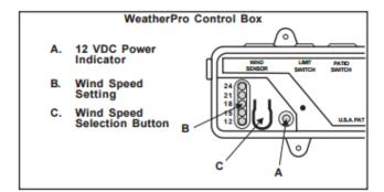
There are six (6) LED's in the WeatherPro control and one button for selecting the wind speed.
