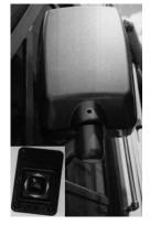
The side exterior mirrors are adjusted by using the multiple directional switches located on the driver's door. Select the mirror to be adjusted by pointing the arrow in the direction of that mirror. Move the control in the direction of movement desired to obtain the best view. The adjustment control moves the top half of both mirrors.
