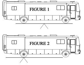
The recommended procedure to weigh a motorhome accurately is on individual corner scales. Since these are not always available, below is a diagram of how to weigh a motorhome on a typical truck scale.
