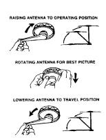
The antenna must be lowered before moving the vehicle. To lower, rotate the directional handle until the pointer is aligned with the pointer on the ceiling plate. Turn the elevating crank (counter-clockwise) in the "DOWN"
