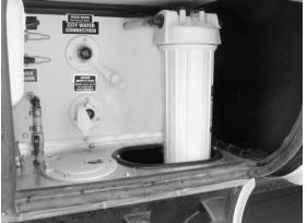
when winterizing your unit. Using the by-pass will keep antifreeze out of the water heater when winterizing the system. Draining the water heater during winterizing is a MUST.
