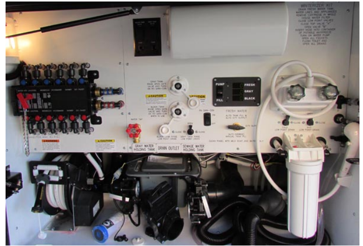
Example of a Water Compartment on a Luxury Coach
