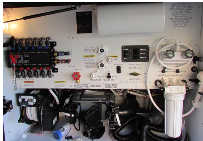
Example of a Water Compartment on a Luxury Coach
