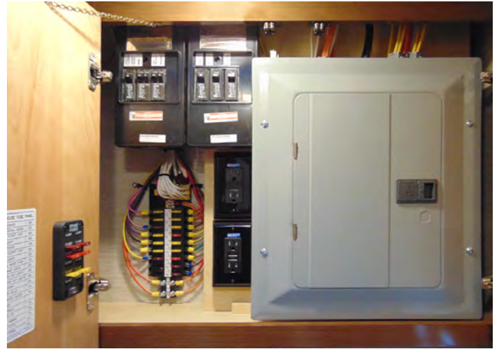
Diesel Pusher Fuse Panel Example
