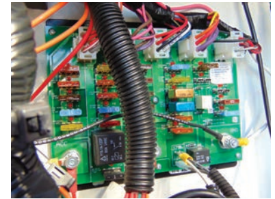
Example of a KIB Fuse Panel
