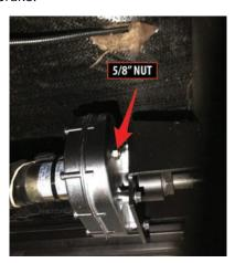
4. Once the brake is removed, use a screw gun or a ratchet with a 5/8" socket to turn the gear reduction nut to retract the slideout.
