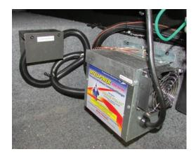
Newmar currently uses three sizes of converters: 45, 60, and 80 Amp models. Previous units may have a 55 or 75 Amp converter or two 45 Amp converters with a total of 90 Amps available. When replacing a converter, it is necessary to use the same size converter to ensure sufficient wiring and breakers for the converter's input and output ratings.
