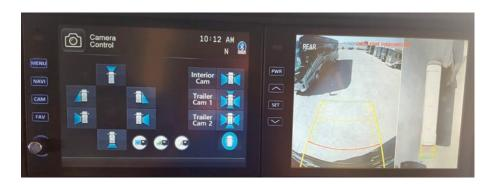
3. The DPGL can be tested by turning the wheel completely in both directions.
