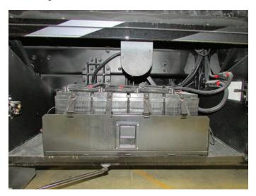
On diesel coaches, the house batteries are normally located in one of the lower compartments. The chassis batteries are normally on the passenger side in the rear compartment on diesel pushers and under the driver's side cab on the front engine on Super C coaches.
