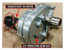
The second option takes longer; however, only a screw gun or ratchet is required. Follow the steps to manually retract the slideout using the gear reduction nuts. This method may be used on both the round and square shaft motors.
