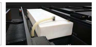
The fresh water tank low point drain valve located in the service compartment near the water hook-up determines whether the city water is going through the water system or into the fresh water tank. The excess water will be vented from an overflow vent pipe onto the ground when the tank capacity has been reached. This pipe is installed in the fresh water tank to prevent tank rupture from overfilling.
