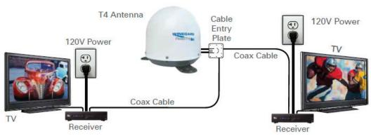
The RoadTrip® T4 antenna switch settings are preset for DIRECTV. If you have a DISH or Bell TV receiver, you must change the numbered switches found on the electronics box under the dome.
