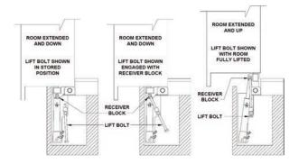
The lift bolt assembly may be mounted vertically or horizontally but will function the same way. Horizontally-mounted lift bolts may not have a cover, depending on the location within the coach.
