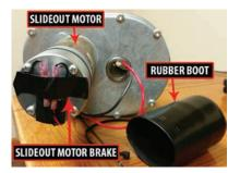
2. Remove the strap, and pull off the rubber boot, removing it from the motor.
