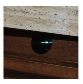
On 2017 and newer coaches, press the push button switch right above the pull-out island to release the island extension. On older coaches, unlock the extension by accessing the lever located in the top drawer.
