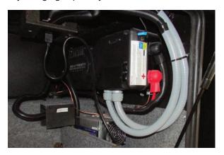
The inverters are usually located in a basement compartment of the coach. Some inverters have a remote panel for an on/off switch in the overhead driver area or above the entry door. When power is supplied by either the generator or shore power, the inverter merely allows the power to "pass through" and will then stop pulling power from the batteries to try and supply 120 Volt power. There is a protective breaker on the inverter to prevent circuit overload.
