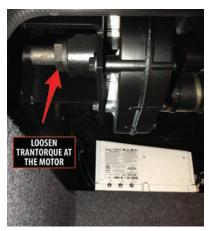
This method requires a significant amount of manpower and is not applicable to the flat floor slide rooms with a square shaft drive motor because there is no trantorque at the motor.
