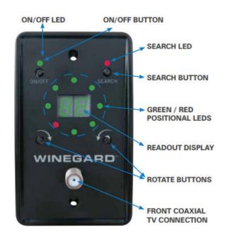
results in the most watchable TV channels. The 2-digit display will show the number of frequencies seen at that position, and both the GREEN and RED LED(s) will be lit to indicate the successful search location.
