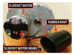
Only a few tools are necessary to complete this procedure; however, it requires the gear box to be operational. Follow the steps to manually retract the slideout by removing the brake and turning the shaft.
