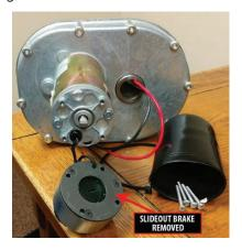
3. Remove the four screws from under the rubber boot on the brake.
