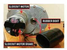
Method three takes longer; however, only a few tools will be needed. This procedure requires the gear box to be operational. Follow the steps to manually retract the slideout using wrench(s).
