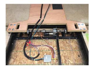
This method is the fastest one if the motor or gears fail, as it does not require battery power. However, this method requires a significant amount of manpower to push in the slideout.
