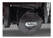
The sewer line must be securely capped during selfcontainment use to prevent leakage of waste material onto the ground or pavement.
