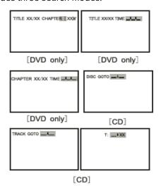
When the above items are showed on LED screen, you can input number to locate desired selector, then press PLAY to commence play. The number you input is invalid if it is beyond the track's capacity.
