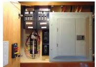
Diesel Pusher Fuse Panel Example
