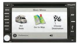
To access the navigation, please select the NAV icon from the Main Menu or tap the NAV button on the front bezel. To exit navigation tap the NAV button again or touch the Audio source icon on the top left of your LCD display. Both these actions will return you to your current audio Source.
