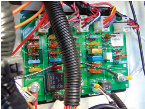
Example of a KIB Fuse Panel
