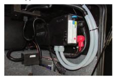
The inverter may provide battery charging while 120 Volts is supplied via the generator or shore power. The inverter performs this action by using the transformer to decrease the voltage and rectify the alternating current into useable direct current voltage. This is regulated by internal sensing circuitry based upon the battery bank's state of charge and several other factors, depending on the coach's particular inverter brand and type.
