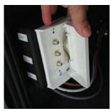
On coaches with a Rayzar automatic TV antenna, this switch is integrated into the power on/off switch typically located in the overhead control center.
