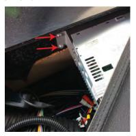
3. Pull the box out of the dash to reach the SD card.
