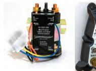
All current Kountry Star, Super Star, Dutch Star, and Ventana diesel coaches use a Precision Circuits all-inone Battery Isolation Manager (BIM). The BIM monitors both the chassis and house battery and is the only place in the coach where they both merge. The BIM only functions when the engine or generator is running or
