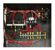
volt circuit breakers that provide power to the house fuse panel, slideout motors, and power awnings.
