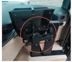
3. Lift up on the chair arm portion, and rotate it approximately 90 degrees. Lower it so the notch aligns with the cross bolt and the micro switch engages. Failure to have seat arm in the correct position will prevent operation.
