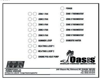
It also contains nine matched pairs of red/green LED's for Zone 1, 2, 3, 4 and 5 Fan(s), Summer Loop, Heat Loop 1, Heat Loop 2, and Engine Pre-heat Pump.
