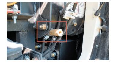
Many coaches also have a connection at the front of the coach under the hood near the generator on the driver side. This connection (on some coaches) will only allow air pressure to be used as a customer connection for external use and will not allow compressed air to enter the system. Coaches plumbed in this manner will have an additional schrader valve port to allow pressurization during production.
