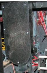
Locate the lift cylinder covers, like the examples shown. Some coaches may have an additional rubber cover installed over the ABS cover to protect the lift from the outside elements.
