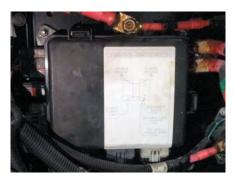
Freightliner Chassis Fuse Panel Example
