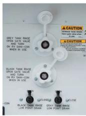
On coaches equipped with tank rinse low point drain(s), turning the tank rinse drain valve to the "open" position will remove pressure and drain the tank rinse line. When finished using the tank rinse, it is recommended to turn off the water supply to the tank rinse connection. Open the valve, and drain off the pressure in the line before disconnecting the water hose.
