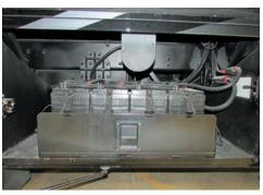
On diesel coaches, the house batteries are normally located in one of the lower compartments. The chassis batteries are normally on the passenger side in the rear compartment on diesel pushers and under the driver's side cab on the front engine on Super C coaches.
