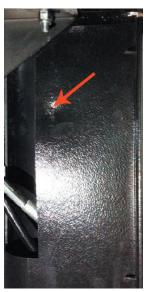
Do not remove the screws on the flat side of the cover. Instead, remove the screws on the side of the cover, allowing the entire cover to be removed. Depending on the location, some covers may be sealed with foam or another sealant.
