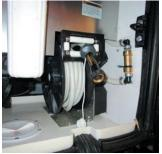
The hose reel deploys manually by pulling the hose outward from the compartment. Once the desired length of hose has been extended, hook up the hose to a potable water source. A switch located on the side of the hose reel requires activation for power retraction. Note: The house battery disconnect must be turned on for the power hose reel to be operated.
