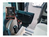
4. Unfold the seat, and rotate the seat down approximately 90 degrees until the pin latch engages in the pin socket.
