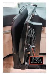
8. Lift the entire seat and support arm, and swivel it approximately 90 degrees to the travel/storage position.
