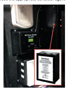
A remote power monitor may be installed in select coaches and allows for continuous visual indication of source voltage and load current or diagnostics.
