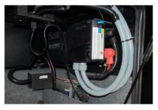
The inverter may provide battery charging while 120 Volts is supplied via the generator or shore power. The inverter performs this action by using the transformer to decrease the voltage and rectify the alternating current into useable direct current voltage. This is regulated by internal sensing circuitry based upon the battery bank's state of charge and several other factors, depending on the coach's particular inverter brand and type.
