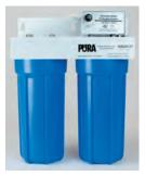
To ensure the Pura filter system operates at optimum level, routine maintenance must be performed. Maintenance and performance depend on water quality and system usage, which will vary by water source. The normal filter life for a Pura filter is four to six months. Clean the system each time the filters are replaced, and disinfect the system at least once per year. Reduced flow rates and deteriorating water quality indicate the filters must be changed.
