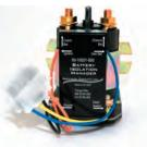
All current Kountry Star, Super Star, Dutch Star, and Ventana diesel coaches use a Precision Circuits all-inone Battery Isolation Manager (BIM). The BIM monitors both the chassis and house battery and is the only place in the coach where they both merge. The BIM only functions when the engine or generator is running or when the coach is connected to shore power.
