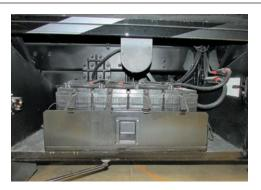
On coaches built on a Ford chassis, batteries are normally located in the front of the coach and can be accessed by opening the hood.
