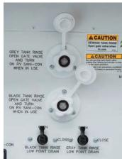
On coaches equipped with tank rinse low point drain(s), turning the tank rinse drain valve to the "open" position will remove pressure and drain the tank rinse line. When finished using the tank rinse, it is recommended to turn off the water supply to the tank rinse connection. Open the valve, and drain off the pressure in the line before disconnecting the water hose.
