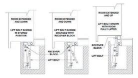
The lift bolt assembly may be mounted vertically or horizontally but will function the same way. Horizontally-mounted lift bolts may not have a cover, depending on the location within the coach.
