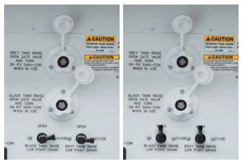
On coaches equipped with tank rinse low point drain(s), turning the tank rinse drain valve to the "open" position will remove pressure and drain the tank rinse line. When finished using the tank rinse, it is recommended to turn off the water supply to the tank rinse connection. Open the valve, and drain off the pressure in the line before disconnecting the water hose.
