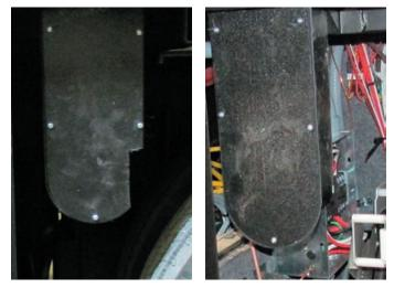
2. Locate the lift cylinder covers, like the examples shown. Some coaches may have an additional rubber cover installed over the ABS cover to protect the lift from the outside elements.
