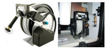
The hose reel deploys manually by pulling the hose outward from the compartment. Once the desired length of hose has been extended, hook up the hose to a potable water source. A switch located on the side of the hose reel requires activation for power retraction. Note: The house battery disconnect must be turned on for the power hose reel to be operated.
