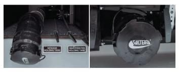
The sewer line must be securely capped during selfcontainment use to prevent leakage of waste material onto the ground or pavement.
