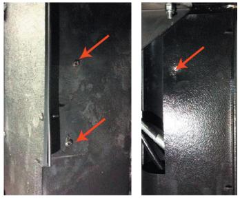
Do not remove the screws on the flat side of the cover. Instead, remove the screws on the side of the cover, allowing the entire cover to be removed. Depending on the location, some covers may be sealed with foam or another sealant.
