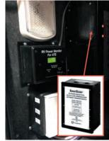
away, the ATS will delay for approximately 2.5 minutes before trying to close the appropriate contactor again.
