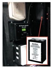
A remote power monitor may be installed in select coaches and allows for continuous visual indication of source voltage and load current or diagnostics. If the ATS fails to close the contactor or transfer when expected, check the 40450 display to see if an error message is displayed. The screen will flash an error message for that failure such as "Loss of Ground", "High Volt", or "Reverse Polarity". The error condition must
