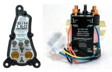
All current Kountry Star, Super Star, Dutch Star, and Ventana diesel coaches use a Precision Circuits all-inone Battery Isolation Manager (BIM). The BIM monitors both the chassis and house battery and is the only place in the coach where they both merge. The BIM only functions when the engine or generator is running or when the coach is connected to shore power.
