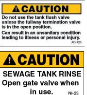
Next, disconnect the freshwater hose and close the gate valve. If there are any solids still left inside the tank, fill the sewage tank with approximately ten gallons of water and holding tank chemical through the stool. As you travel, the agitation of the water should help liquefy any solids left in the tank. You can dump the sewage tank again at your next destination.
