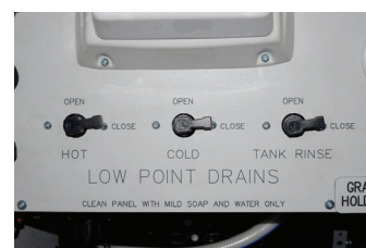
Low Point Drain Configuration Examples
