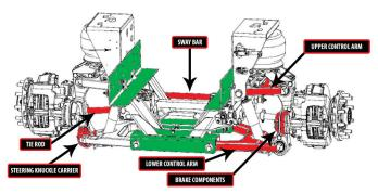
The chassis frame and suspension cradle (shown in green) are the proper lift points for towing.
