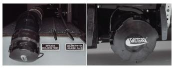
The sewer line must be securely capped during selfcontainment use to prevent leakage of waste material onto the ground or pavement.
