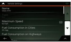
Fuel consumption and engine type information is used to calculate and estimate amount of fuel needed as well as the approximate of CO2 produced. Also changeable for larger vehicle profile types are the "Extended Vehicle Settings."
