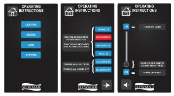
Touch the ON button to turn on the selected light circuit. Touch the OFF button to turn off the selected circuit. On lighting circuits with dimming capability, drag the slider to adjust the brightness of the selected light circuit.
