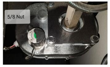
5. After the slideout is fully retracted, reinstall the brake.
