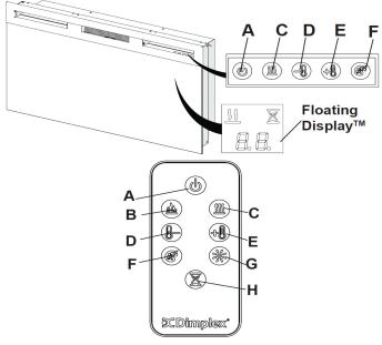
The unit can be controlled by either the manual controls which are located on the upper right of the fireplace or the remote. The fireplace is supplied with an IR multifunction remote control.
