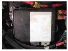
Freightliner Chassis Fuse Panel Example
