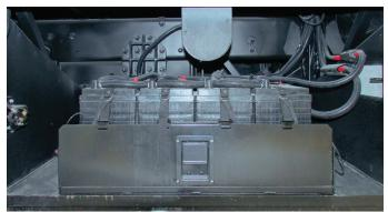
A battery wiring label is located inside the battery compartment and shows how the batteries are wired together. Replacement batteries must be wired according to the diagram shown. Replacement batteries should be of the same brand and capacity as the originals.
