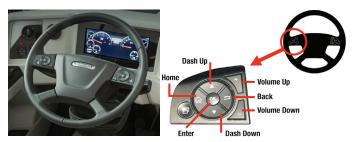
Starting with the 2023 model year, select Freightliner coaches (Kountry Star, Ventana, Dutch Star, New Aire) have the steering effort factory-set on the Favorites menu on the Valid Glass Dash menu. The setting can be adjusted using the up and down arrows without scrolling through the Glass Dash menus.
