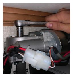
On the left-hand motor, turn the bolt counterclockwise to retract the room on the left side. Turn the bolt clockwise to extend the room on the left side.
