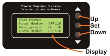
(Note: 50A Service or Generator Service overrides the SET Button.) If there have not been any key presses for awhile, the PCS monitor turns off the backlighting to save on power. The first press of any key will only turn on the back lighting.
