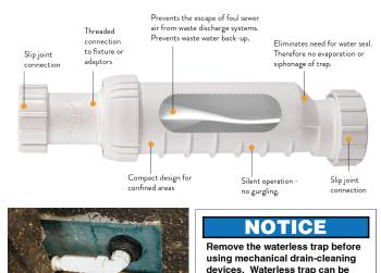
Foreign objects, such as hair, in the trap may allow odor to enter the coach and impede or slow water drainage and require occasional cleaning. When removing the waterless trap for cleaning, the ridges must be down and the direction of water flow must be correct when re-installed.
