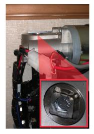
To retract the slideout, reach over the fascia using a ratchet and socket. Place it on the bolt head, and turn the bolt. As the bolt is turned, the slideout will begin to move.
