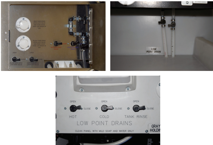
Low Point Drain Configuration Examples
