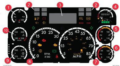
NOTE: This instrument cluster is shown with the U.S. speedometer, which shows miles per hour (mph) more prominently than kilometers per hour (km/h).
