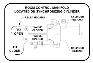
1. Determine which synchronizing cylinder controls the room. Manually open the valve release cams for the extend and retract solenoid valves by moving the cams to the "valve opened" position as shown.
