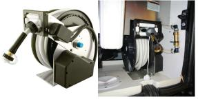
The hose reel deploys manually by pulling the hose outward from the compartment. Once the desired length of hose has been extended, hook up the hose to a potable water source. A switch located on the side of the hose reel requires activation for power retraction. Note: The house battery disconnect must be turned on for the power hose reel to be operated.
