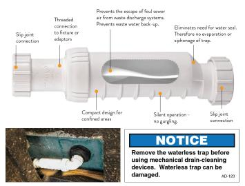
Foreign objects, such as hair, in the trap may allow odor to enter the coach and impede or slow water drainage and require occasional cleaning. When removing the waterless trap for cleaning, the ridges must be down and the direction of water flow must be correct when re-installed.
