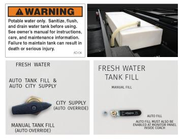
The fresh water fill valve located in the service compartment near the water hook-up determines whether the city water is going through the water system or into the fresh water tank. The excess water will be vented from an overflow vent pipe onto the ground when the tank capacity has been reached. This pipe is installed in the fresh water tank to prevent tank rupture from overfilling.
