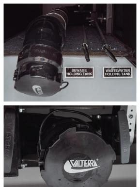
The sewer line must be securely capped during selfcontainment use to prevent leakage of waste material onto the ground or pavement.
