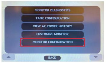
10. Using the down arrow, scroll to the last page of the MONITOR CONFIGURATION screen. Then select the REBOOT button.
