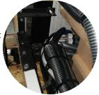
from within the slideout to the rest of the plumbing in the coach. This hose easily moves with the slideout as it extends and retracts. The plumbing lines are normally tied to the flexible drain pipe and extend and retract smoothly as the slideout travels.
