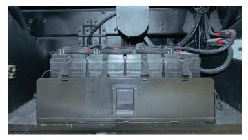
On diesel coaches, the house batteries are normally located in one of the lower compartments. The chassis batteries are normally on the passenger side in the rear compartment on diesel pushers and under the driver's side cab on the front engine on Super C coaches. On coaches built on a Ford chassis, batteries are normally located in the front of the coach and can be accessed by opening the hood.
