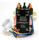
All current Kountry Star, Super Star, Dutch Star, and Ventana diesel coaches use a Precision Circuits all-inone Battery Isolation Manager (BIM). The BIM monitors both the chassis and house battery and is the only place in the coach where they both merge. The BIM only functions when the engine or generator is running or when the coach is connected to shore power.
