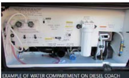
EXAMPLE OF WATER COMPARTMENT ON DIESEL COACH
