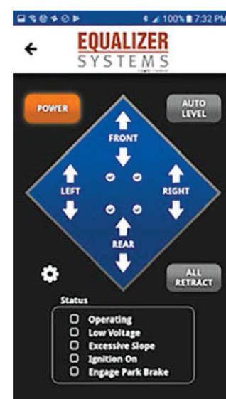
Power & Jack Down lights are illuminated during and after this process
