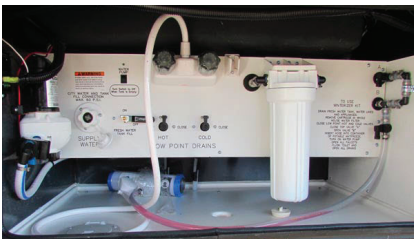
EXAMPLE OF WATER COMPARTMENT ON GAS COACH
