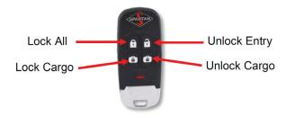
Pressing a button on the FOB should cause the LED to flash multiple times. The LED will also flash anytime it is located by an antenna. This happens when you start your vehicle and the FOB search near the driver's seat is initiated. The FOB is powered by a standard 2032 3V battery.
