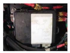
Freightliner Chassis Fuse Panel Example
