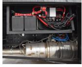
certain parameters are met, the BIRD, BIM, or charge bridge will activate and allow charge to the chassis battery. This prevents the chassis batteries from being drained by the interior 12 volt equipment and allows ample voltage for engine ignition.
