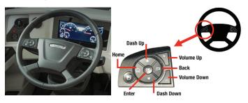
Starting with the 2023 model year, select Freightliner coaches (Kountry Star, Ventana, Dutch Star, New Aire) have the steering effort factory-set on the Favorites menu on the Valid Glass Dash menu. The setting can be adjusted using the up and down arrows without scrolling through the Glass Dash menus.
