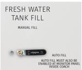
The fresh water fill valve located in the service compartment near the water hook-up determines whether the city water is going through the water system or into the fresh water tank. The excess water will be vented from an overflow vent pipe onto the ground when the tank capacity has been reached. This pipe is installed in the fresh water tank to prevent tank rupture from overfilling.
