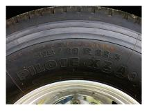
This tire size is 315 / 80 R 22.5. From this size, we can determine the physical dimensions of the tire, as well as its basic construction. The tire size breaks down like this:
