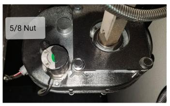
5. After the slideout is fully retracted, reinstall the brake.
