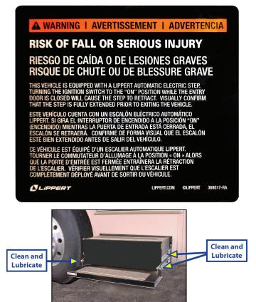
Source(s): Kwikee by Lippert Components 47 Series Electric Step Owner's Manual (3010001164) Rev 07.13.18
