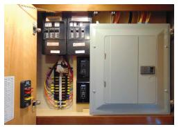
Diesel Pusher Fuse Panel Example
