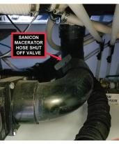
• The macerator is designed to process human waste and toilet tissue, making the Sani-Con ideal for black water, as well as gray water, discharges.
