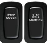
In addition, select coaches are equipped with step treads that can be lifted for additional storage. Some coaches may also have a switch that operates the step well lighting.
