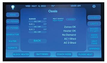
The Oasis control screen can only be accessed from the Climate All screen and allows the user to control the Oasis Hydronic Heating system burner and both hydronic heating system electric heating elements.
