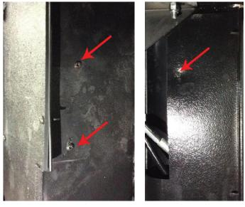
Do not remove the screws on the flat side of the cover. Instead, remove the screws on the side of the cover, allowing the entire cover to be removed. Depending on the location, some covers may be sealed with foam or another sealant.
