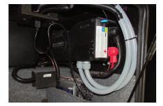
The inverters are usually located in a basement compartment of the coach. Some inverters have a remote panel for an on/off switch in the overhead driver area or above the entry door. When power is supplied by either the generator or shore power, the inverter merely allows the power to "pass through" and will then stop pulling power from the batteries to try and supply 120 Volt power. There is a protective breaker on the inverter to prevent circuit overload.
