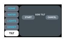
holding tank slope angle to aid in dumping the holding tanks. This feature was first implemented during the 2023 model year on London Aire, Essex, and King Aire coaches.
