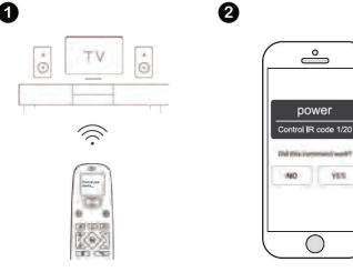
Keep U1 Line-of-Sight with your device, click Power first, then choose Yes or No to see if it works. During the process, the U1 remote control will emit infrared signals to the device. And U1 will be able to find the proper code set after searching database.
