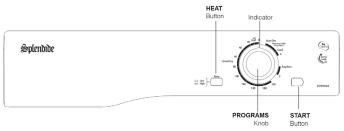
The START button begins drying a selected program. The HEAT button selects drying temperature:
