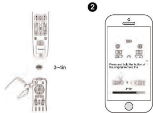
Keep U1 Line-of-Sight with your original remote, select the icon of the function key that needs to be copied. Meanwhile, long press the corresponding function key of the original remote. If the App notifies you it's successful, it means it's completed. If not, please try again.
