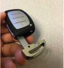
2. Insert tip of mechanical key into front section of slot and gently twist to separate FOB case.
