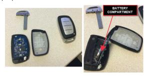
4. Reassemble & gently snap both sides of FOB together. Insert mechanical key fully into slot until it snaps in place.
