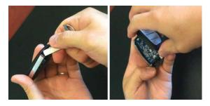
3. Access battery compartment & remove old battery. Replace with new CR2032 battery & install in proper orientation as shown.
