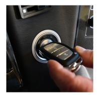
Use the lock button end of the Smart Key Fob to contact the engine START/STOP button directly. A single press of the engine START/STOP button with the Smart Key Fob will change as follows:
