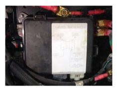
Freightliner Chassis Fuse Panel Example
