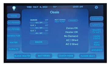
The Oasis control screen can only be accessed from the Climate All screen and allows the user to control the Oasis Hydronic Heating system burner and both hydronic heating system electric heating elements.
