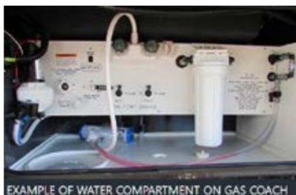
EXAMPLE OF WATER COMPARTMENT ON GAS COACH
