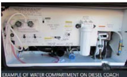
EXAMPLE OF WATER COMPARTMENT ON DIESEL COACH
