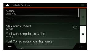
Fuel consumption and engine type information is used to calculate and estimate amount of fuel needed as well as the approximate of CO2 produced. Also changeable for larger vehicle profile types are the "Extended Vehicle Settings."
