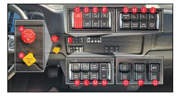
Dash-mounted switches are backlit to illuminate the text and icon on the switch. Press the upper half of the switch to turn the desired lamp(s) on or off. If the lights have a dimming function, hold the switch down to cycle the light between bright and dim.
