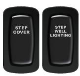
In addition, select coaches are equipped with step treads that can be lifted for additional storage. Some coaches may also have a switch that operates the step well lighting.
