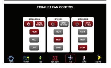
Touch the FANS icon to jump to the Exhaust Fan Control page. Select which fan you wish to operate and press the power button. Once the power button turns red, power is supplied to the selected fan location. The buttons are gray while the circuit is inactive. The available buttons will vary by coach model and floorplan, as well as installed options, and may include, but are not limited to:
