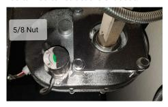
3. After the slideout is fully retracted, reinstall the brake.
