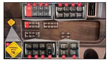
Dash-mounted switches are backlit to illuminate the text and icon on the switch. Press the upper half of the switch to turn the desired lamp(s) on or off. If the lights have a dimming function, hold the switch down to cycle the light between bright and dim.
