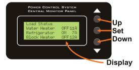
(Note: 50A Service or Generator Service overrides the SET Button.) If there have not been any key presses for awhile, the PCS monitor turns off the backlighting to save on power. The first press of any key will only turn on the back lighting.
