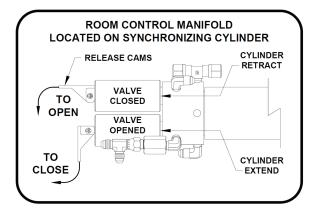
Determine which synchronizing cylinder controls the room. Manually open the valve release cams for the extend and retract solenoid valves by moving the cams to the "valve opened" position as shown.
