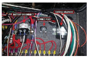
Most of this power flows through the battery disconnect to the fuse block or mini-breakers, which prevents overloading the circuit prior to progressing to the 12 Volt load. There are some 12 Volt circuits that do not go through the house battery disconnect; however, these loads still pass through a fuse or mini-breaker before progressing to the load.
