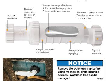
Foreign objects, such as hair, in the trap may allow odor to enter the coach and impede or slow water drainage and require occasional cleaning. When removing the waterless trap for cleaning, the ridges must be down and the direction of water flow must be correct when re-installed.
