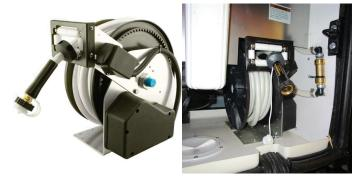
The fresh water system in the coach is designed to operate at a maximum of 60 PSI. Water pressure levels above this level can damage the fresh water plumbing in the coach. If the water pressure ever surpasses 60 PSI, a pressure regulator must be installed to reduce the incoming pressure, or fill the fresh water tank and use the internal water pump to supply water to the coach.
