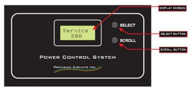
The Midi-PCS will constantly monitor 120VAC RV power and shed and restore power to the five controlled loads. The display panel has all the brains, a data connector to the I/O module, and an additional connector to control the air conditioners through low voltage signals. The I/O Module houses a current sensor, two relays to control 120VAC powered appliances, and Service Type detect circuitry.
