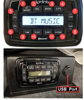
Phone Charging Capability: The USB input can be used for charging most phones. A successful charging will be manifested by the battery indication status on the phone itself. In addition, the PRV250 will also note "USB CHRG."
