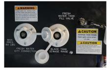
To disconnect from the city water supply, close the valve from the water supply. Release the pressure by rotating the fresh water valve to the tank fill position. Remove the hose from the city water supply, and store it in the water compartment. Once the pressure is relieved, rotate the fresh water valve to the appropriate operating position.
