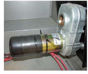
Depending on the year, model, and floorplan of the coach, the exact slideout motor(s) location may vary. Generally, they may be accessed from under the slideout in the compartment area. Some motors may also be located in the wheel well area under a cover.
