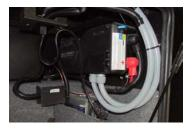
**Inverter/Converter Combinations:** Many Newmar coaches are equipped with inverter/charger combination units, sometimes referred to as inverter/converter units. These units range from 1200 to 3000 watts and serve as a three-stage charger and an inverter. Coaches equipped with this option will also be equipped with a 120 Volt subpanel.
