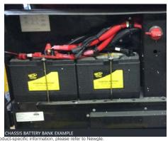
The type and brand of chassis battery may vary depending on coach year, make, and model. Chassis batteries may need to be disconnected and removed from the coach to maintain proper electrolyte levels or perform routine battery maintenance. House batteries may be either serviceable Liquid Lead Acid/Flooded or AGM/Sealed Cell.
