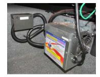
**Inverter/Converter Combinations:** Many Newmar coaches are equipped with inverter/charger combination units, sometimes referred to as inverter/converter units. These units range from 1200 to 3000 watts and serve as a three-stage charger and an inverter. Coaches equipped with this option will also be equipped with a 120 Volt subpanel.
