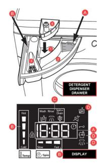
**Section B:** In section B, pressing the corresponding button allows you to view the maximum spin speed and temperature values attained by the machine during the set wash cycle, or the values selected most recently, if these are compatible with the set wash cycle.
