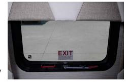
In the event of an emergency, open the window: Remove the screen by pulling out on the red handle. Push and release the lever from the locking hook. Rotate the lever 90 degrees, and push it through the slot in the window frame. Escape through the opening.
