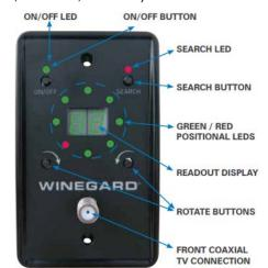
Turn the power switch on for the antenna. Within 10–15 seconds, the dish will begin moving and should make one or two revolutions during startup. During this process, it is normal to hear a slight grinding sound as the unit checks its rotational limits. This does not harm the unit. The system will pause to acquire GPS.
