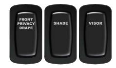
The Visor switch is located on the dash and adjusts the windshield screen up or down. When the ignition switch is turned on it limits the visor travel to approximately 1/2 way down and with the key off it travels all the way down to the dash. The screen will travel up until it reaches the stop setting.
