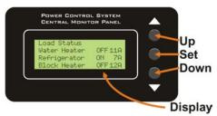
(Note: 50A Service or Generator Service overrides the SET Button.) If there have not been any key presses for awhile, the PCS monitor turns off the backlighting to save on power. The first press of any key will only turn on the back lighting.
