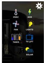
HVAC: The HVAC icon displays the controls for the rooftop air conditioners, furnace, or Oasis hydronic heating system, and provides access to the HVAC settings for the entire coach.
