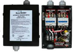
Transfer switches are designed so that only one input can be connected at a time in order to prevent any backfeeding of electrical power. In addition, RV transfer switches generally have a built-in delay allowing the generator to warm up and speed up before actually switching the load. This prevents stalling or stumbling while the engine is still cold and not producing full power.
