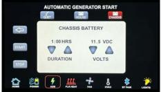
Notes: When there is a demand for the generator to run or stop, there can be up to two minutes of delay. During this time, the AGS is checking if there are any other demands.
