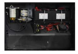
The chassis batteries are recharged by the vehicle's electrical system whenever the engine is running. With an added charge bridge solenoid or BIM, the vehicle's charging system will also charge house batteries if parameters are met.
