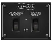
**Electric Bedroom Slideouts:** The operating switch for the bedroom slideout is usually located on the bedroom wall. If there is a full wall slideout on the driver side of the coach, the switch may be located on the wall that separates the bedroom from the living room.
