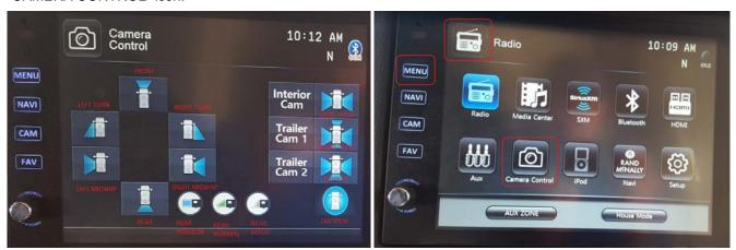
When first starting the engine: The camera monitor should display the REAR NORMAL view when first starting the engine.
