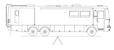
To find the total weight of the unit, pull the unit onto the scales so that all of the wheels are on the scale as shown. Record the weight. This is the GVW and should not exceed the GVWR supplied by Newmar for the unit.
