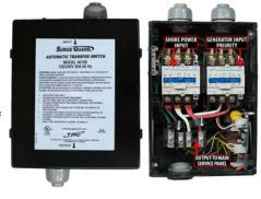
Transfer switches are designed so that only one input can be connected at a time in order to prevent any backfeeding of electrical power. In addition, RV transfer switches generally have a built-in delay allowing the generator to warm up and speed up before actually switching the load. This prevents stalling or stumbling while the engine is still cold and not producing full power.
