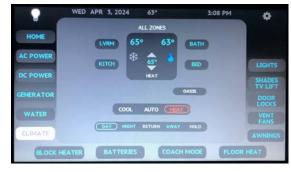
**Heat & Cool Buttons**: Press the Heat or Cool button to activate all the zones at one time. This will make the user unable to set heat in one zone and air conditioning in another at the same time.
