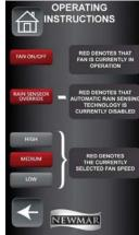
fan speed (High, Medium, or Low). A red button indicates the fan is currently in operation, which fan speed is selected, or the automatic rain sensing technology is disabled.
