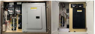
On a diesel pusher coach, the house fuse panel, which controls most of the components and appliances inside the coach, is located in the bathroom, front overhead next to the 120 volt breaker panel, or the rear wardrobe. This panel contains fuses and breakers that are connected to the main appliances in the coach, from the refrigerator and television to the lights in the bedroom and slideouts.
