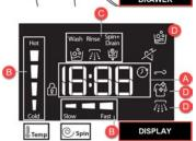
**Key Lock:** To lock the control panel, press and hold the "Key lock" button for approximately 3 seconds. The symbol will light up on the display to indicate that the control panel has been locked (with the exception of the "ON/OFF" button). This prevents unintentional changes to programs, especially with children near the machine. To unlock the control panel, press and hold the "Key lock" button for approximately 3 seconds.
