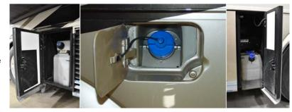
Some vehicles are equipped with a remote DEF fill-port. If so equipped, the remote port is directly opposite the DEF tank on the other side of the vehicle, and has a blue cap over the fill-port. DEF parts, such as the fill cap or tank, are
