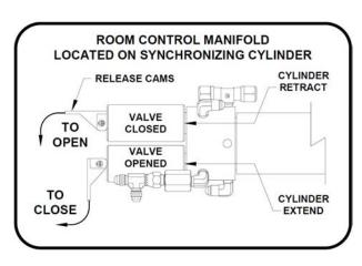
If the pump manifold is equipped with an auxiliary hand pump, you may be able to retract the room by opening only the room retract valve (as labeled by the wiring harness) and operating the hand pump, refer to the "Auxiliary Hand Pump Operation" page (in your HWH Operator's Manual) for instructions on the use of the hand pump and valves equipped with a release cam. If the room cannot be retracted with the hand pump, it will be necessary to use the lift bolts and room retract screws.
