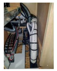
The drain lines connecting slideout-installed components, such as the kitchen sink and other optional equipment utilizing the coach water supply, are typically hard-plumbed within the slideout. The hard plumbing from the kitchen slideout connects to the hard plumbing from the tank using a braided drain line to ensure flexibility as the slideout extends and retracts.
