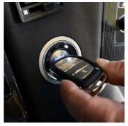
Press and hold the engine **START/STOP** button
