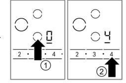
If there is no cookware on the cooking zone, the cooking zone display blinks. This means that the cooking zone tries to detect the cookware. Place cookware on the cooking zone within 30 seconds, or the cooking zone will switch itself off.
