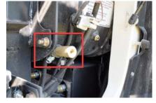
When using air from the connection, the engine should be running to operate the compressor. The air pressure is regulated by the air governor for the chassis air system. The approximate pressure can be monitored by the gauges on the dash. The air connections are supplied and plumbed by the chassis manufacturer.
