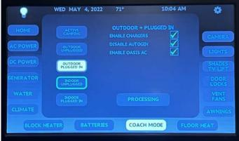
**Indoor Unplugged:** When the motorhome is stored indoors while unplugged, press the Indoor Unplugged button, followed by the Activate button. This will automatically provide a list of items that should be enabled or disabled.
