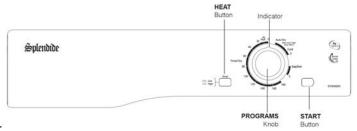
The PROGRAMS knob sets the program: rotate it clockwise, never counter-clockwise, until the indicator is pointing to the program you want to select. The programs knob will advance to the '0' position after the program ends.
