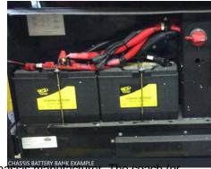
The chassis batteries on your motorhome are installed and warranted by the chassis manufacturer. The coach (or house) batteries on your motorhome are installed by Newmar Corporation, but warranted by the battery manufacturer. These batteries are used to operate the 12 volt items that are not a direct part of the chassis.
