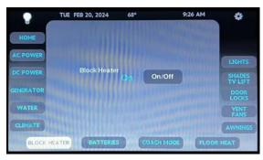
Press the On/Off button to toggle the block heater's electrical circuit on or off. The current status displays beside the button (ON, OFF, SHED).
