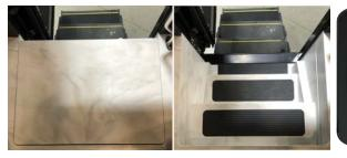
On select coaches, the switch for the interior step cover is located either on the side of the passenger console, on the dash console near the center, or near the mid-entry step well. Press the switch forward to extend the step cover to make it level with the coach floor. Press the switch backward to lower and retract the cover in the stored position.
