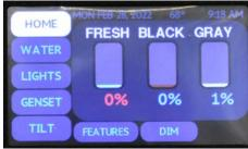
**Tank Status (Tank Monitoring):** The fresh, gray, and black holding tank statuses are displayed as percentage-full levels. These values are displayed as both a numerical percentage and a bar graph.
